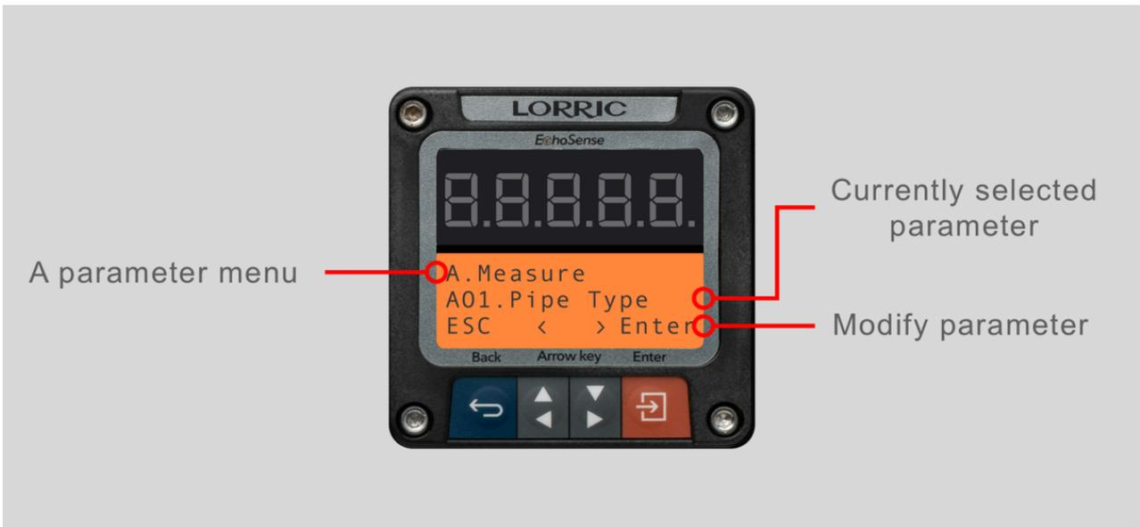
If there is a N/A on the lower right corner of an option, it means that this version of the hardware does not have this function, and you cannot enter the option.
