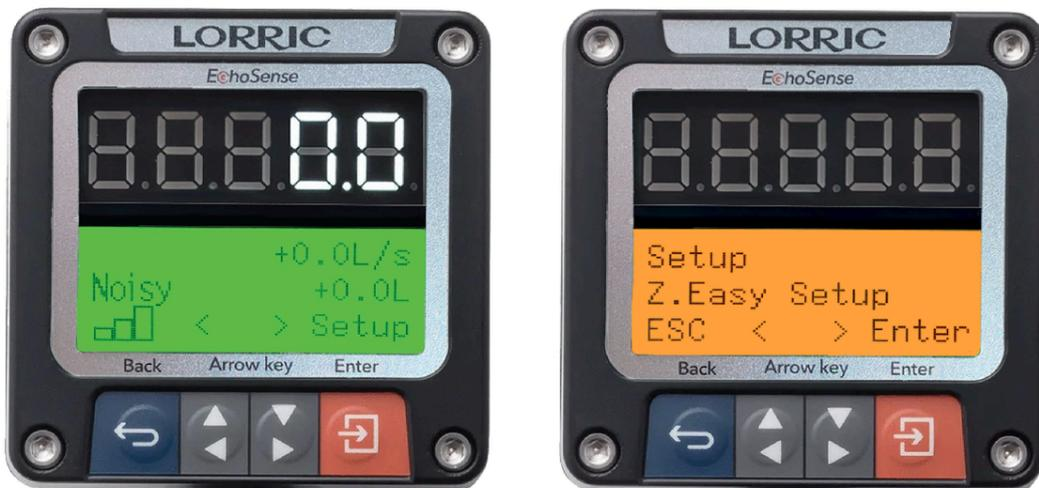
2. **Settings Page:** In the "(Z Quick Menu)" options interface, locate and select the "(Z02 Automatic Pipe Size Detection)" menu, then press enter.
